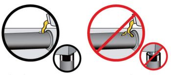
Only fill pump to recommended level, and fill only when the connected cylinder is fully retracted.
